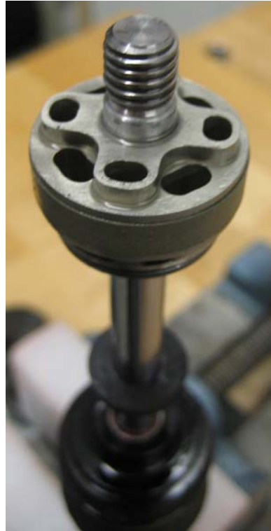
Correct piston orientation
