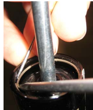
Remove circlip
