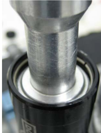
Cane Creek Adaptor with circlip installed
