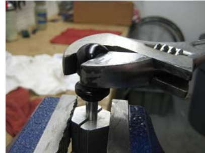
Remove end eye with adjustable wrench
