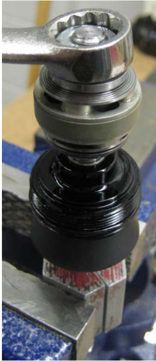
Remove shaft nut
