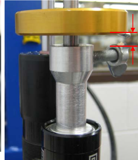
Set IFP depth at 5mm from cylinder head
