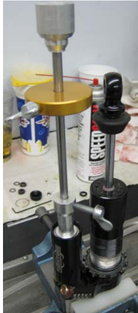
IFP Setting Tool installed
