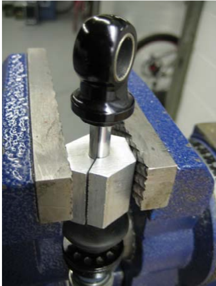
Shaft in shaft vise
