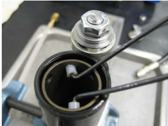
Pull out inner tube
