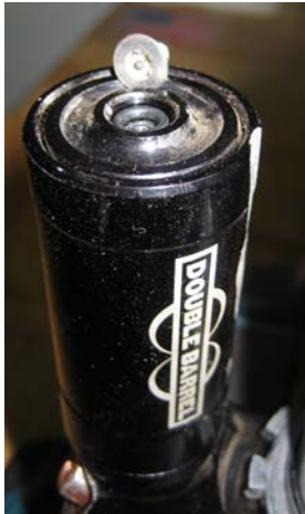
Remove Torx Screw
