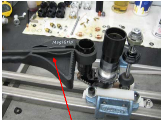
IFP o-ring IFP wrench IFP glide ring Strap wrench
