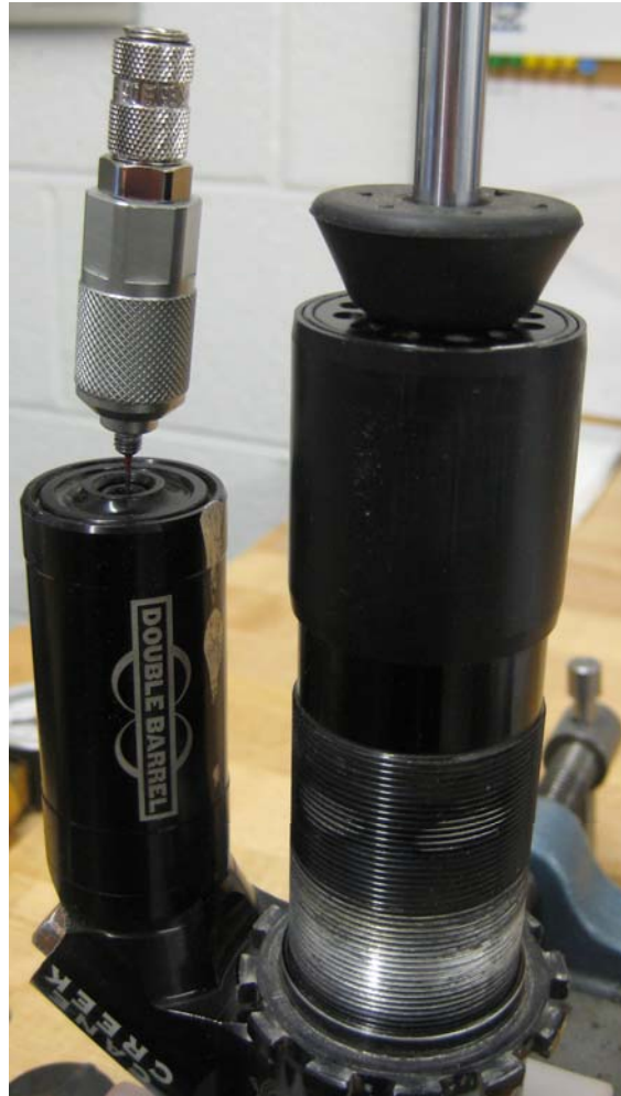
Drain pressure from reservoir
