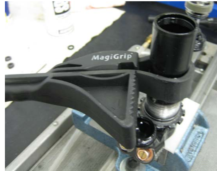
Strap wrench on outer tube
