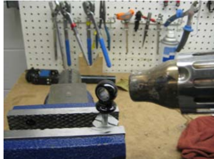
Heat gun used to free Loctite
